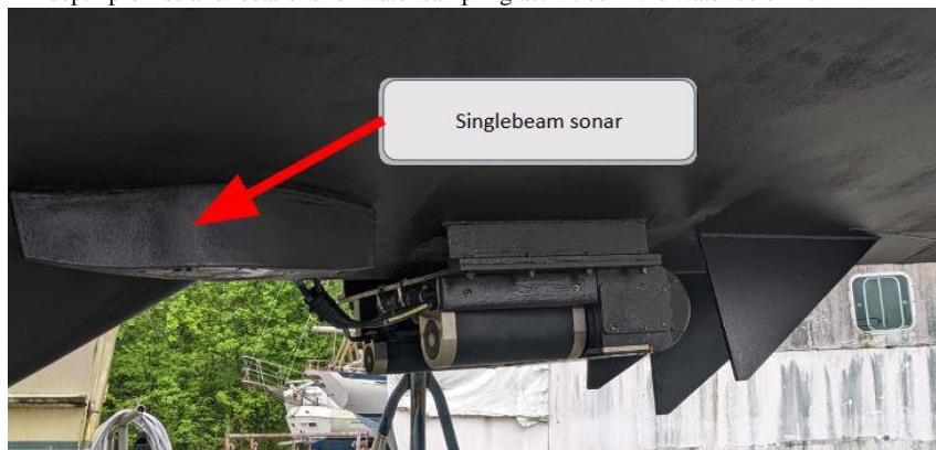
Figure 8 Singlebeam Sonar location (starboard hull)
