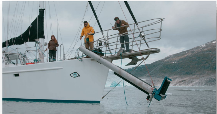
Figure 2 ORP & MTG team deploy R2Sonic on USM Megatower aboard SRV Marie Tharp
